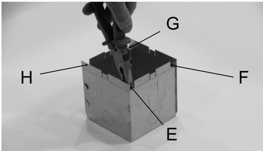
Bend the 4 tabs E-F-G-H inwards at 90° in order to prepare a support for the plaster spotlight.
