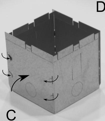
Fold sides C and D 90° and insert the protruding tabs into the proper slots; bend them to firmly close all sides.
