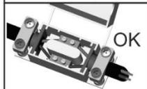
CONNECT CABLES BY INSULATED TERMINAL BOX, WITH CABLE CLAMPS ON BOTH SIDES (not included)
